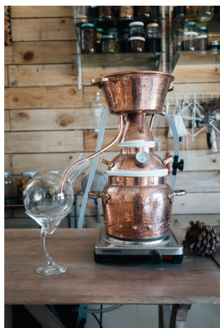
An alquitar still (with an innovative collection set up) in our Alembics Lab © Peter Rees Photography
